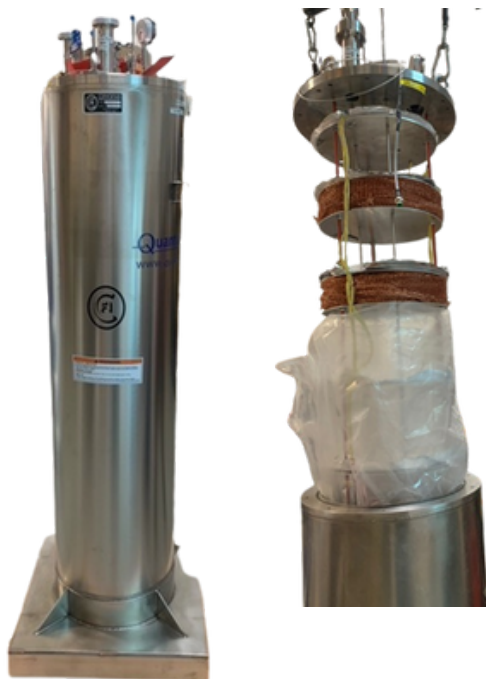
Cryostat & cryostat internals
