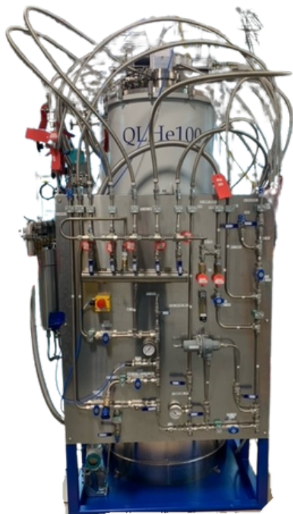
QLHe100 Quantum Helium / Hydrogen Liquefier 100L/day
