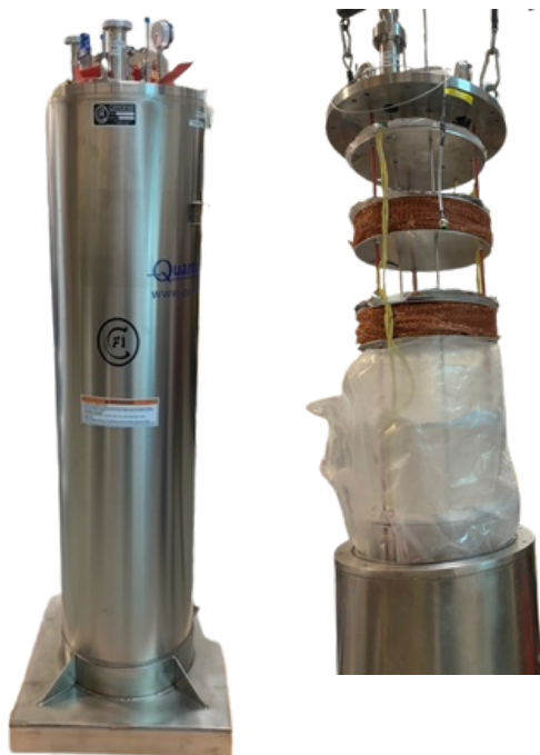
Cryostat & cryostat internals
